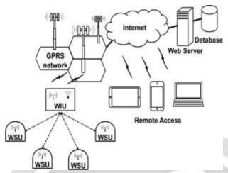
Fig1: Configuration of the automated irrigation system. WSUs and a WIU based on microcontroller, ZigBee, and GPRS technologies.
