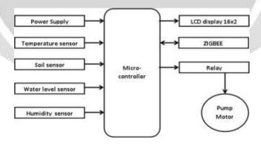
Fig2.Wireless Sensor Unit
