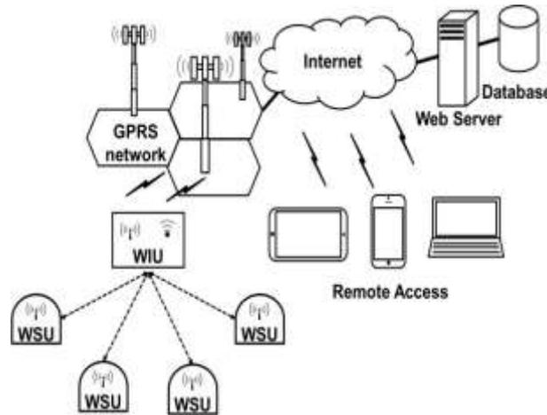
Fig1: Configuration of the automated irrigation system. WSUs and a WIU based on microcontroller, ZigBee, and GPRS technologies.
